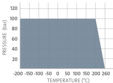
The temperature and pressure recommendations in the graphs apply to gaskets 2.0 mm thick that are used with raised face flanges. Higher stresses are possible when thinner gaskets are used! The information provided must therefore be considered as estimates that are on the safe side rather than as specific operational limits.
